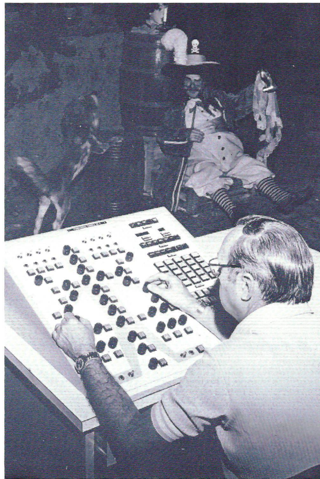
One of the last steps before shows are assembled for the EPCOT pavilions is programming of Audio-Animatronics characters. Console above has knobs to adjust movements of limbs and face. (Copr. Walt Disney Productions)
